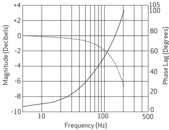
Measured with 40 % signal amplitude, at 3,000 psi (210 bar) pilot or operating pressure, fluid viscosity of 24 cSt, and fluid temperature of 104 °F (40 °C)
